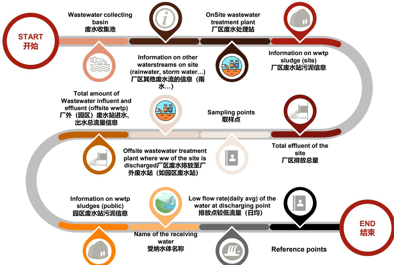
A simple waste effluent flow chart should show all relevant wastewater streams. The flow chart should contain the given information.
