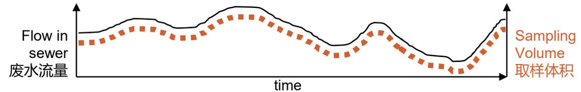
**Volume-proportional** → a constant sample volume at variable time intervals according to the wastewater volume is drawn
