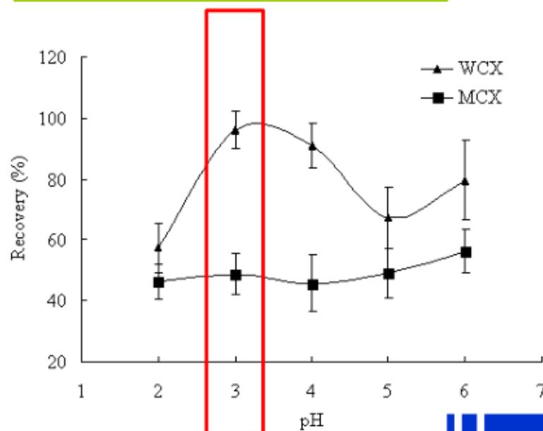
Recoveries of ofloxacin in WCX and MCX cartridges at different pHs of loading solution (error bars indicate the standard deviations, n = 3)
