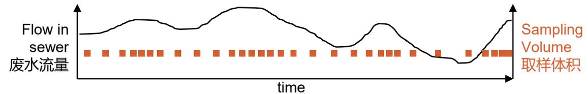
**Spot sample** → a defined sample volume at a specific time is drawn. 特定的时间取规定体积的样品。
