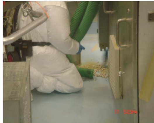
Back-to-back cleaning - press Korsch 3 - disconnecting hoses with tablets
