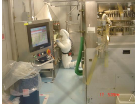
Back-to-back cleaning - press Korsch 3 - vacuuming filter housing
