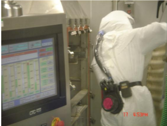
Back-to-back cleaning - press Korsch 3 - removing pre-filters
