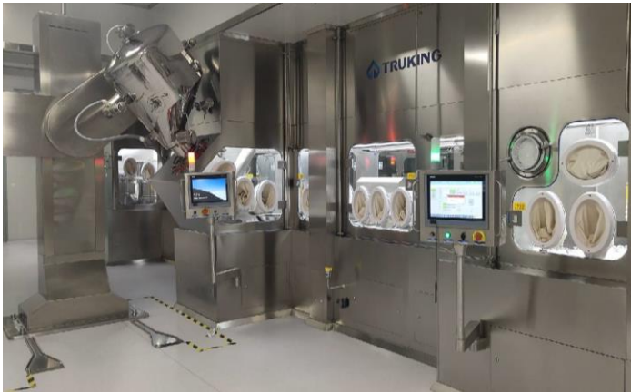
Automatic packing in rigid isolator
