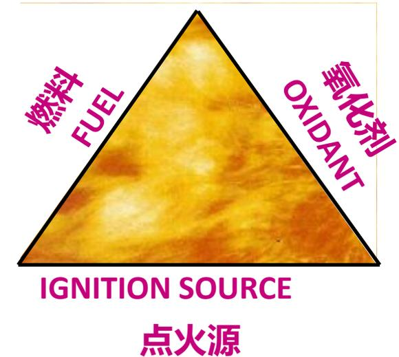
**Fuel + Oxygen = Flame + Heat + Gaseous Combustion Products**
