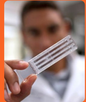
Example of a Kinetic Chromogenic LAL or rCR Cartridge. Source: Charles River Laboratories
