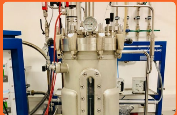
Reactor holding cell culture for manufacturing recombinant proteins such as rFC.
