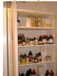
Flammable liquids in wood cabinets
