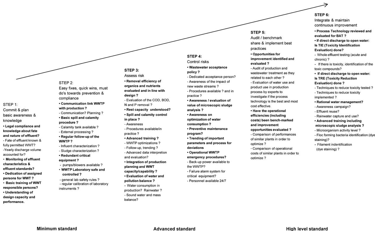
Figure 1. Wastewater maturity ladder. BAT=best available techniques; BOD=biochemical oxygen demand; COD=chemical oxygen demand; WWT=wastewater treatment; WWTP=wastewater treatment plant.
