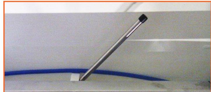
Door closed **AND** shaft not fully in position "filter clamped" !
