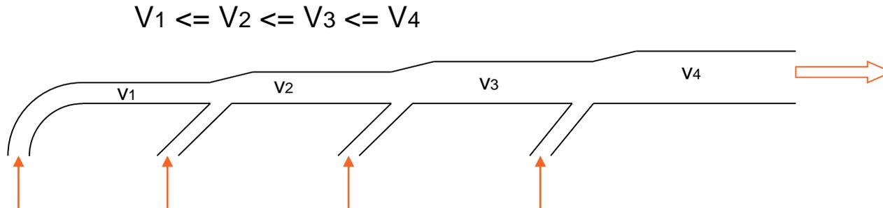
The duct diameter is changed step wise to maintain or slightly increase velocity towards the end. Velocity shall never be allowed to decrease.
