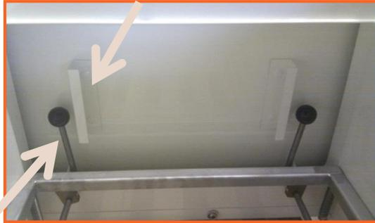
Shaft position "filter clamped"
