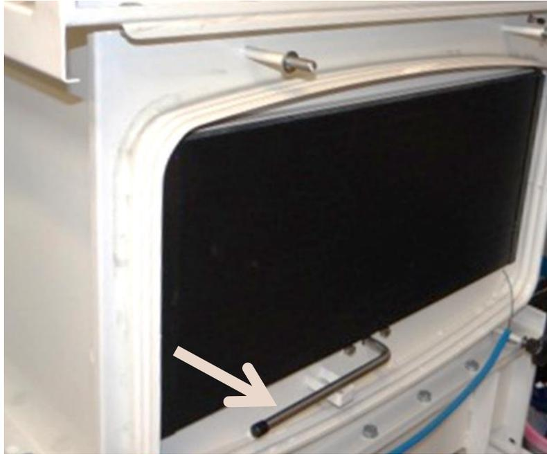
Shaft position "filter clamped"
