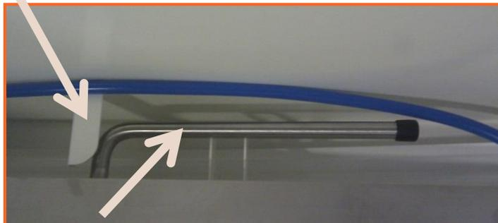
Shaft position "filter clamped"
