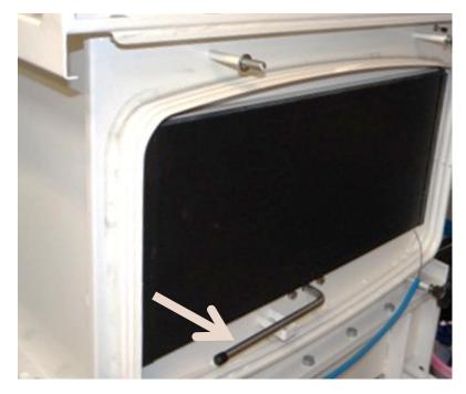
Shaft position "filter clamped" BUT filter not fully sealed
