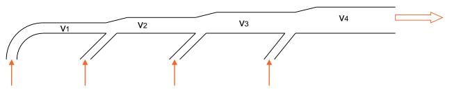
The duct diameter is changed step vise to maintain or slightly increase velocity towards the end. Velocity shall never be allowed to decrease.
