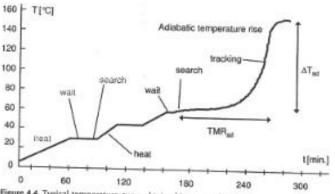
Figure 4.4 Typical temperature curve obtained in an accelerating rate calorimeter using the heat, wait, and search mode.
