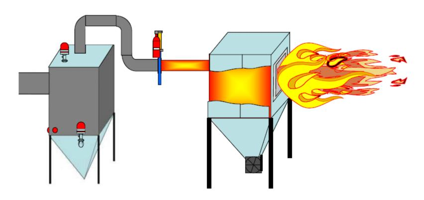
If the Kst is above 300 bar.m/s, the valve would not work
