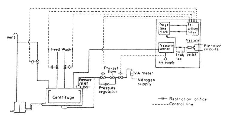
Figure 2. Schematic drawing of pressure-monitored inerting system (for batch centrifuge).
