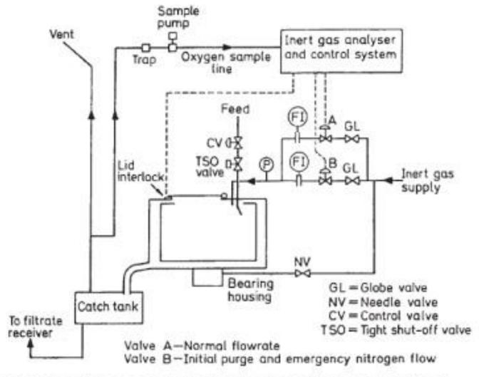
Figure 3. Schematic drawing of oxygen-monitored inerting system (for batch centrifuge).
