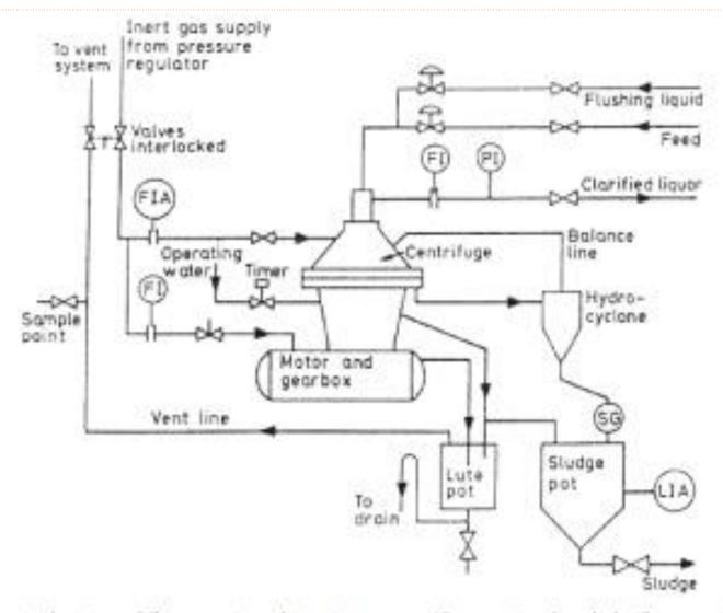
Figure 1. Schematic drawing of flow-monitored inerting system (for opening bowl clarifier centrifuge).
