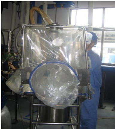
Operation outside isolator 隔离器外
