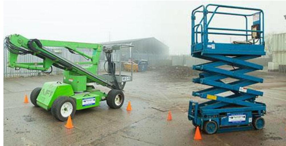
Mobile Elevated Work Platform (MEWP)
