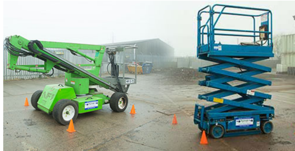
Mobile Elevated Work Platform (MEWP)
