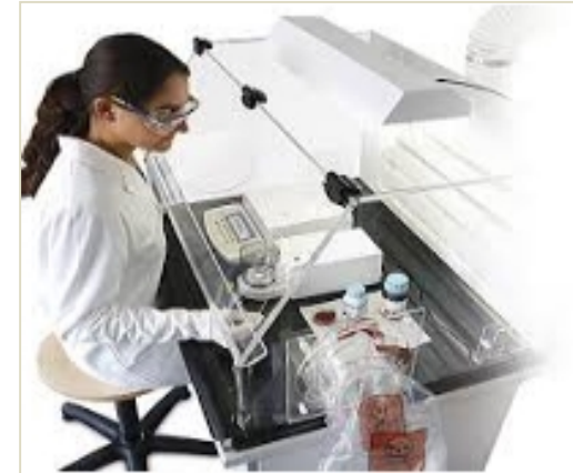
Ventilated Enclosure Cabinet for Weighing
