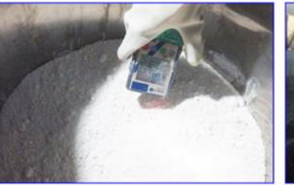
14. Checking the static voltage of material.
