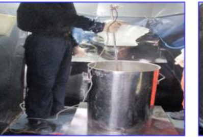
15. Arranging Multi static discharge Rod into material.
